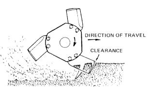
Correct blade setting showing clearance at back of blade.
