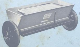
H. The Acre Soil Shredder driven from the Merry Tiller is capable of handling turf, peat, moss, bulb fibre, etc. to a continuous output of approximately 2 cubic yards per hour.
