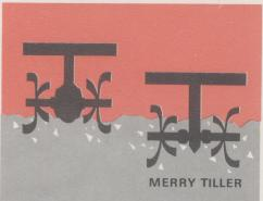
Deeper tilling depth: A Merry Tiller digs in deep—a full 12" down. Most worm-gear tillers can't go nearly that deep because their bulky transmission housings keep them shallow. But Merry Tiller's thin transmission case knifes right in and works for you.
