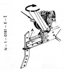
The handle column is twisted into place. The pedal for sideways adjustment is held down until the correct position is reached. The throttle lever box is pressed into place in the slot on the front of the handle column. Check the movement of the lever. Make sure there are no sharp kinks in the cable and try the lever to see that it moves evenly and easily. Mount the arrester bar using the arrester bar bolt (A).
