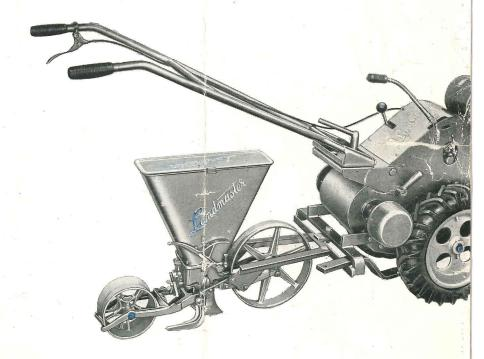
The "LANDMASTER" Seed Drill fitted to the Tool Bar of the Tractor. The Seeder has a capacity of 19 pints and the flow of the seed is controlled by a single lever. The Seeder will sow from the smallest seeds up to peas and beans (French).
