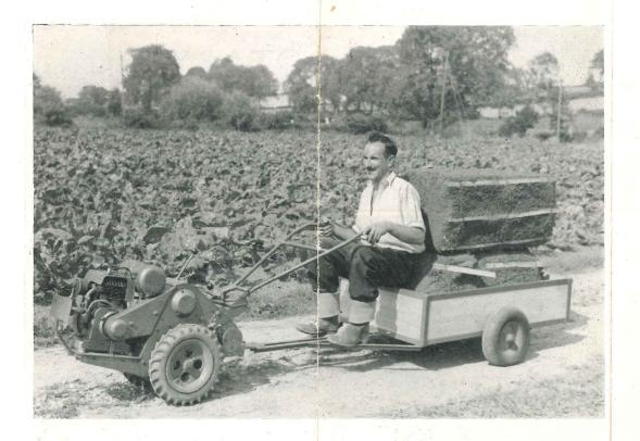
The Trailer is steel framed with timber body and is mounted on 16"x 4" pneumatic wheels.
